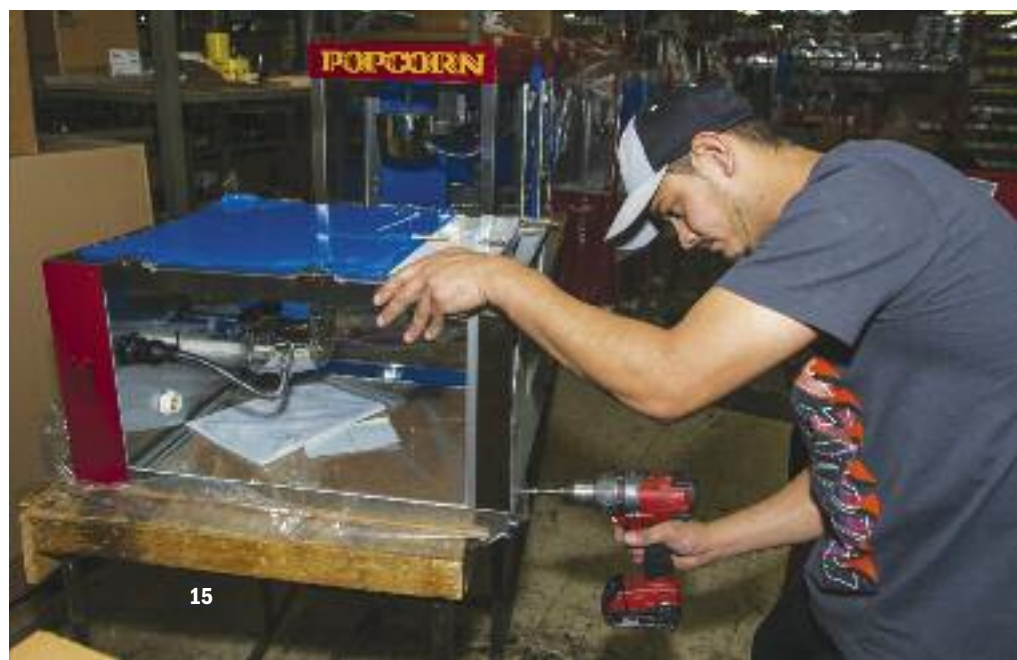
C. Cretors & Company employee Danny Sotelo assembles a popcorn machine at the company's manufacturing facility.
